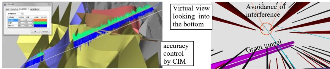
Figure 12. Quality control on drilling by information modeling system
