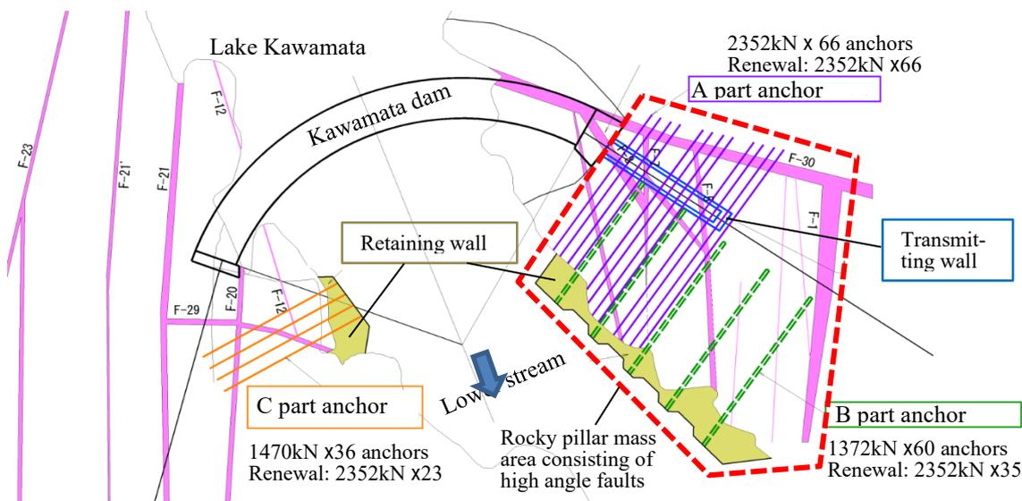
Figure 1. Plan of Kawamata Dam, transmitting wall and PS anchors in rock foundation
