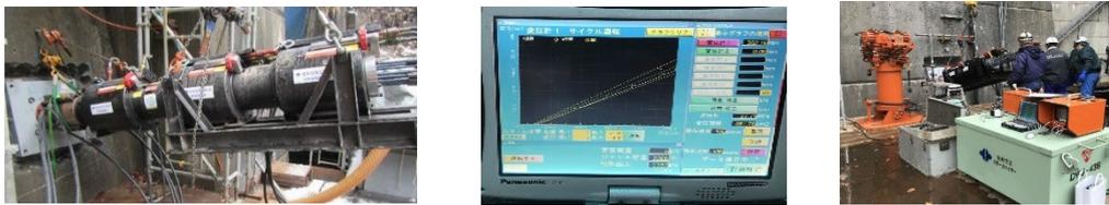
Figure 13. Triple coupled large tension jacks and tension control system
