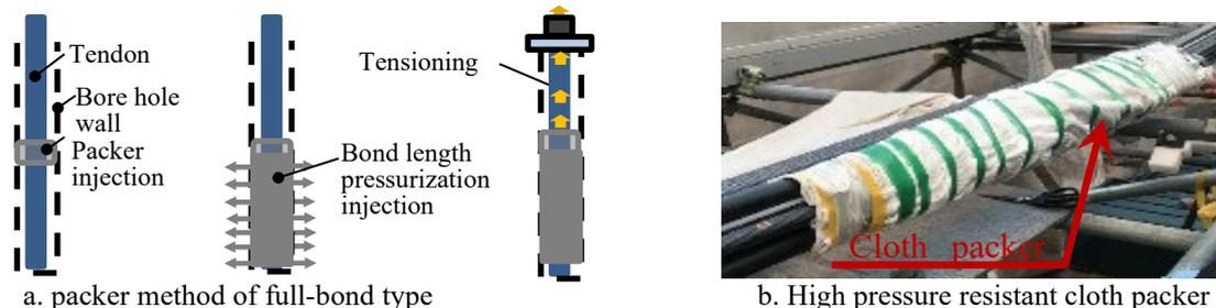
Figure 15 Development of cloth packer on full bonded type anchor
