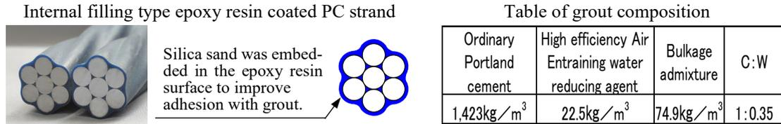
Figure 4. Anti-corrosion protection by ECF strand and super high-quality grout
