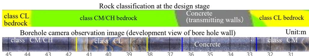
Figure 11. Bore hole wall confirmation diagram by underwater borehole camera system
