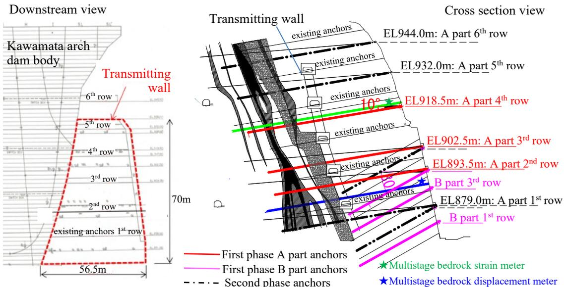
Figure 2. Downstream view and Cross section view of left bank on PS anchors and transmitting wall
